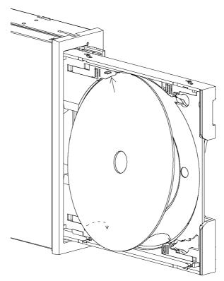
4. Check three disc holders to confirm to the disc surely.
